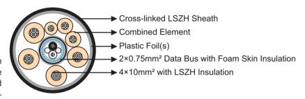
• UIC Data Bus 0.75mm<sup>2</sup>: Two foam skin insulated tinned copper stranded conductors are twisted together with two filling elements to a pair.
