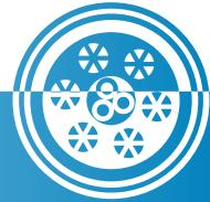
Multi cores: All cores natural coloured, printed with numbers, starting in center with number 1.
